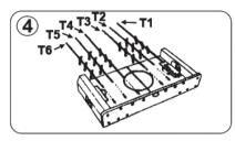
Insert the metal bars(T1,T2,T3,T4,T5 and T6) into the designated holes in the long panel.
