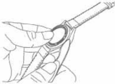
step 1. use an open knife to open the case back
