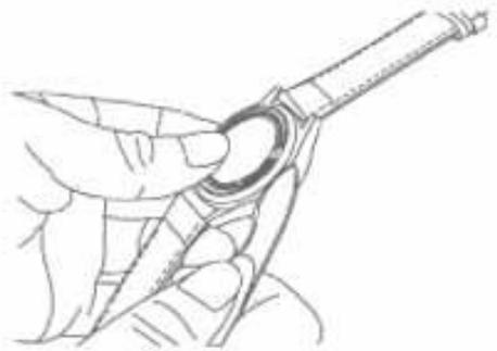
step 1. use an open knife to open the case back
