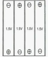
Open the battery cover and install 4pcs 1.5V AA batteries (not included) according to the +/- polarity as indication inside as above image.
