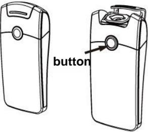
1. Push open the cap, the LED around the button will turn on.
