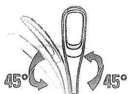
The neck of the lamp can rotate horizontally (right/left) within a 90-degree angle (45 degrees to the left and 45 degrees to the right).
