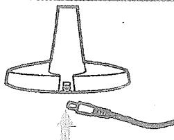
Connect the adaptor into the rear hole of the lamp base and insert the plug in a socket.
