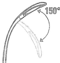
The neck of lamp can be adjusted vertically (up/down) within a 150-degree angle.
