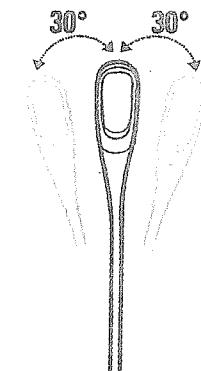
The head of the lamp can be adjusted sideways (right/left) within a 60-degree angle (30 degrees to the left and 30 degrees to the right).
