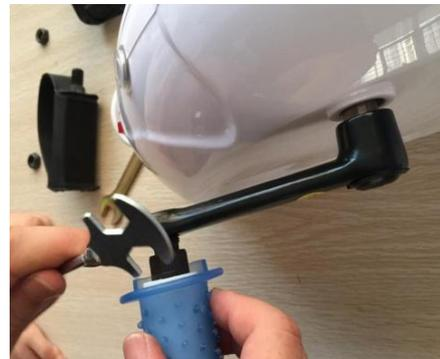
4. Turn the threaded rods in the right and left pedal holder with the aid of a screw wrench until the thread is screwed completely.
