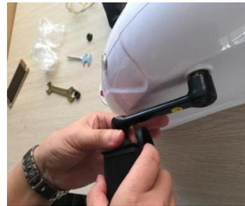
3. Please screw the nuts with the screw wrench at the ends of the threaded rods, while fixing the pedals with another screw wrench.
