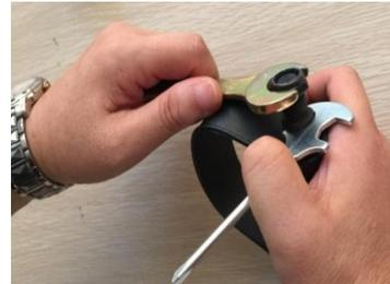
2. Turn them with a screw wrench through the mouths, while holding the screw wrench directly at the strong tightened nuts at the pedals.
