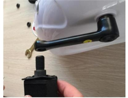
2. Screw both pedals out of the holders and place the handles ready. They are marked with "L" and "R" at the threads ends for left and right.
